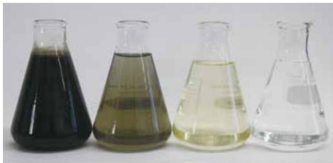
Sewage and septic tank sludge Dewatering separation liquid Biologically treated water Discharged water
